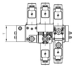
• đ Φ  $\oplus$  Valve section 2 with 4/3-way directional spool valve type NBVP16 (NG6), flow pattern symbol G, with additional elements, orifice Ø0,8 and check valve in port P (coding /B0,8R), restrictor check valve in ports A, B (coding ABR2,0/BBR1,5), pressure switch type DG3 for port A, Pressure gauge till 400 bar for port B (coding /A3B9/400) and return pressure stop (coding /S) mounted onto sub-plate (coding /0). Valve section 3 with directional spool
